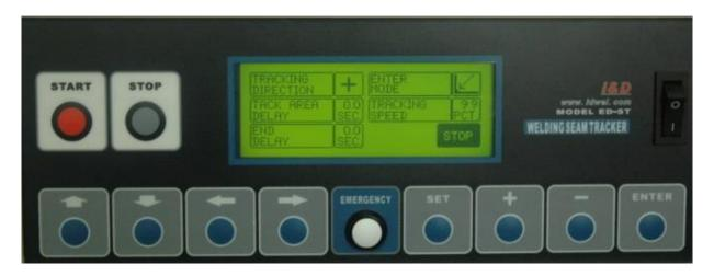
The Tracking controller front panel has a LCD display and the basic operation keys.
